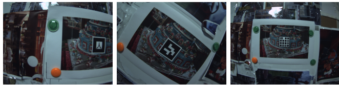
Fig. 7. Sample images from the dataset. Images are from Seq #1 (with ARToolKit), Seq #2 (with AprilTag 25h9) and Seq #3 (with TopoTag) from left to right respectively.
