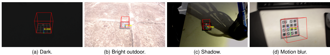
Fig. 18. TopoTag detection in different real scene tests with a rolling shutter camera. (Best viewed in color)
