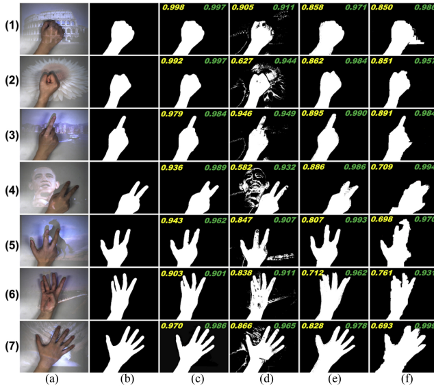
Fig. 13. Visual comparison. (a) Original image. (b) Ground-truth. (c) Our method. (d) SCM [30]. (e) BkSub [32]. (f) GB [33]. The yellow (top-left) and green (top-right) numbers in each result image are the corresponding precision p and recall r values, respectively.
