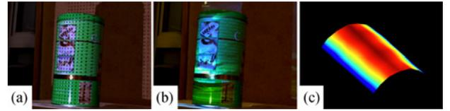
Fig. 18. Comparison experiment on sensing cylinder object. (a) GSL illumination. (b) ISL illumination. (c) Reconstruction result of ISL.
